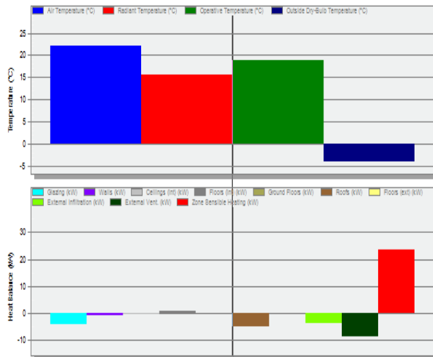
Figure 7. Thermal analysis obtained based on the second modeling of the city of Manchester
